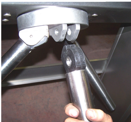
1. Seat the arm on the rotor
