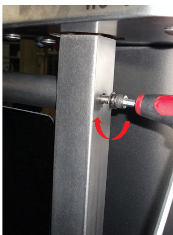
2. Tighten top fixing screw
