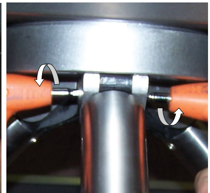
3. Tighten screws with 5 mm. keys
